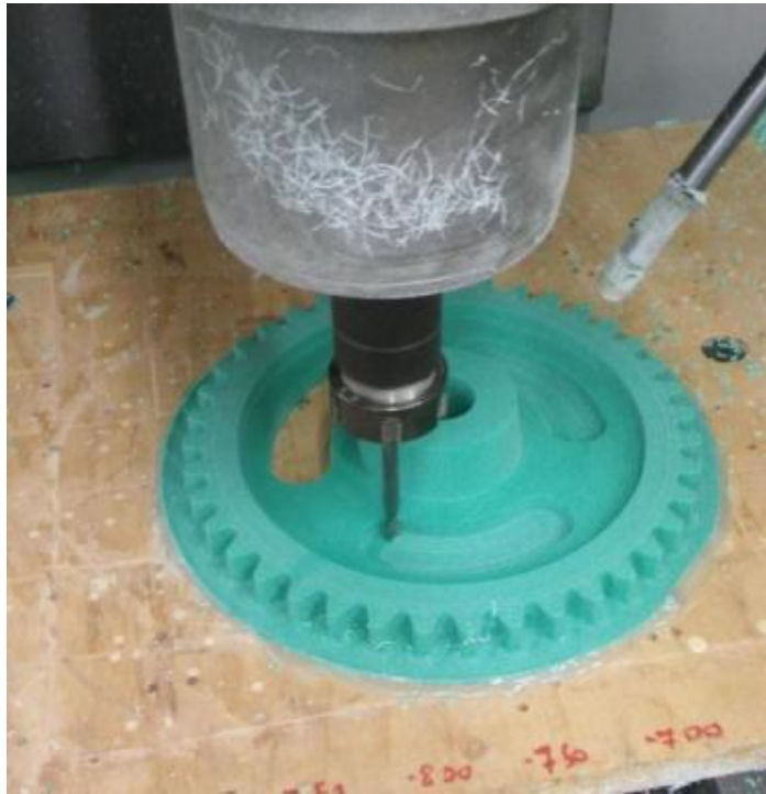
Fig. 6 – Gear slot production
