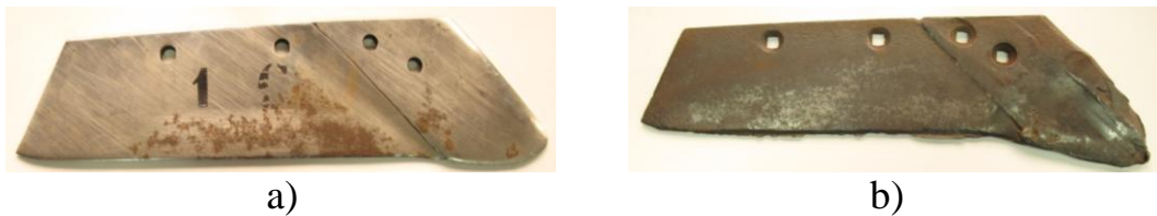
a) standard ploughshares “A”; b) welded ploughshares „B“ on additional material S355JO
