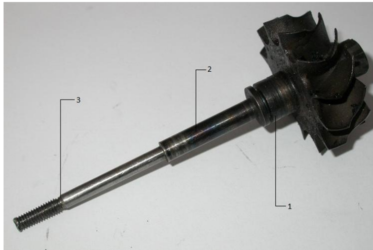
Fig. 9 Colors change on different sections of the axle
