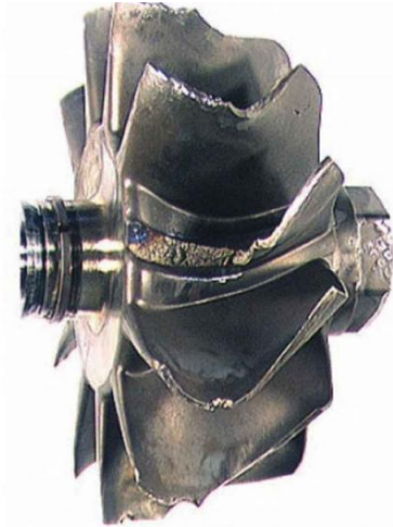
Fig. 1 The representation of damaged of the rotor blades [5]
