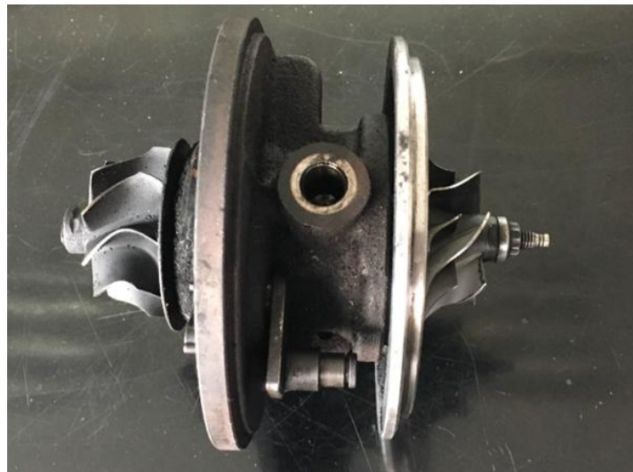
Fig. 6 Visual inspection of the inner parts of turbocharger
