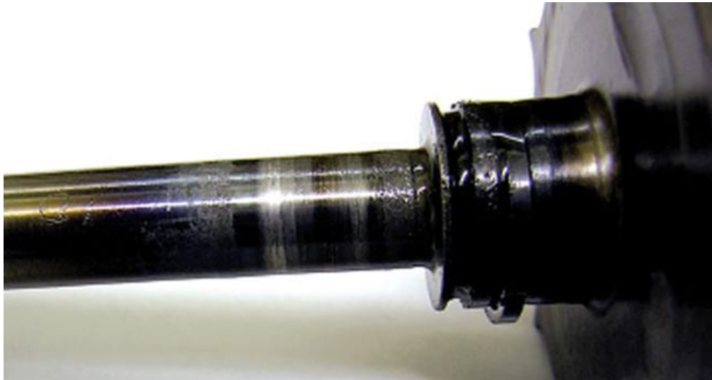
Fig. 3 The representation of color change on the turbocharger axle [5]
