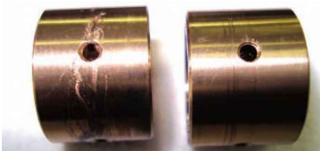
Fig. 2 The representation of damaged of the sliding bearing [5]
