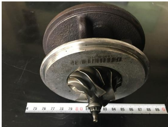
Fig. 8 Visual inspection of compressor blades
