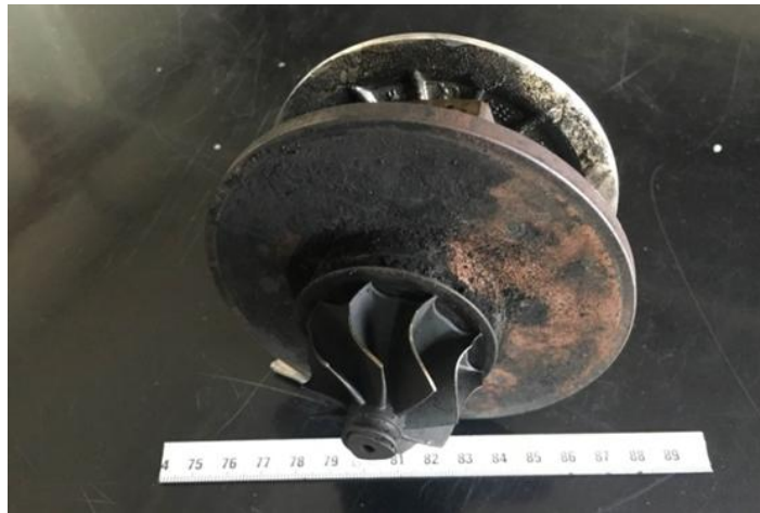
Fig. 7 Visual inspection of turbine blades
