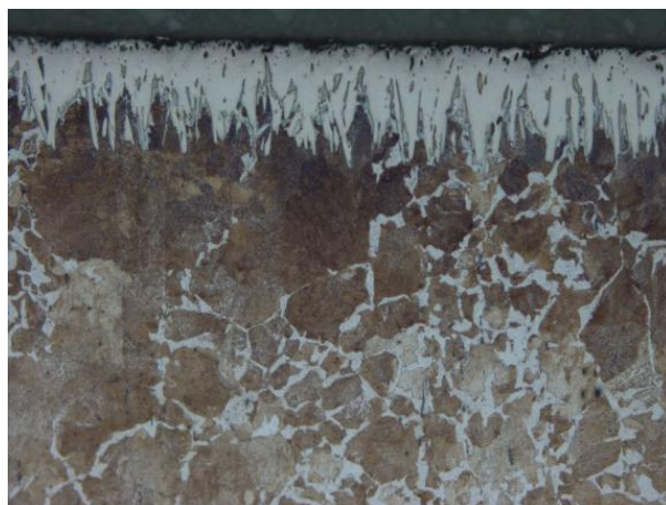
Fig. 2 Microstructure of obtained boride layer
