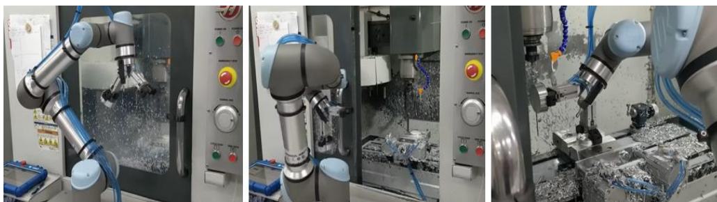
Figure 2. Collaborative robot UR5 during the execution of loading and unloading operations of workpieces on a CNC machine tool in a digitalized production environment
