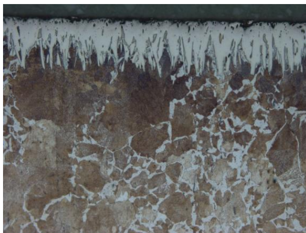
Fig. 2 Microstructure of obtained boride layer
